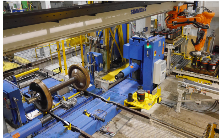
A programmable robot grasps a bearing to be pressed onto a wheel set.
